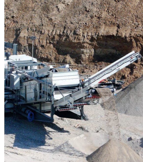
3-Deck Siebmaschine 1800 x 6000 mm
