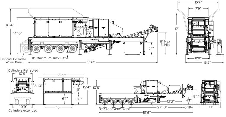
Feeder module shown with optional hydraulic lift system.
