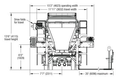
Jnit shown with the following options: extended walkway along chutes, hydraulic power for roll-away chutes, removeable switchgear panel, and 4 crank jacks.
