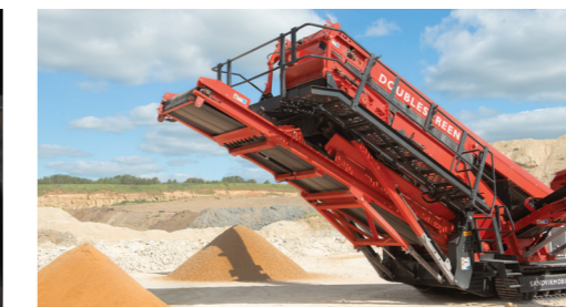
Three sided walkway around main conveyor
