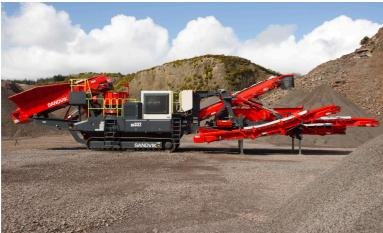
$Featuring \ the \ proven, high \ performing \ Sandvik \ CH430 \ Hydrocone. \ Available \ with \ optional \ double \ deck \ hanging \ screen \ system.$
